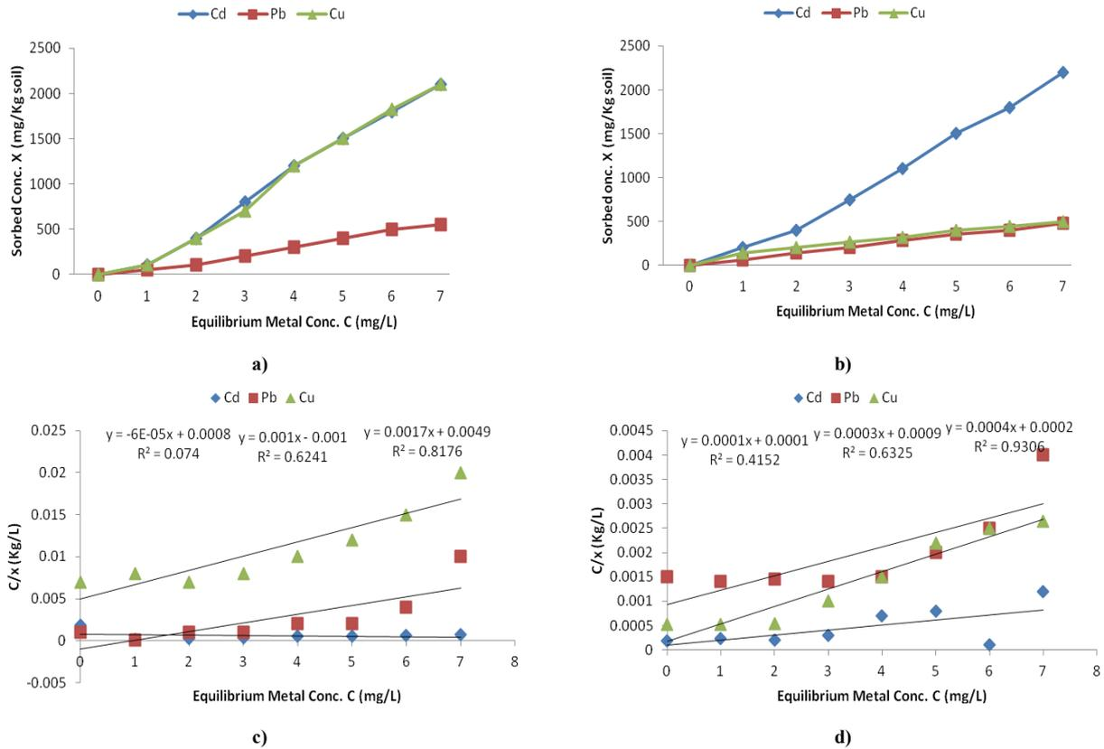
Fig. 4. a) Sorbed conc. of metals on Gujranawala soil; b) Sorbed conc. of metals on Shahdara soil; c) Langmuir isotherm of metals on Gujranawala soil; d) Langmuir isotherm of metals on Shahdara soil
