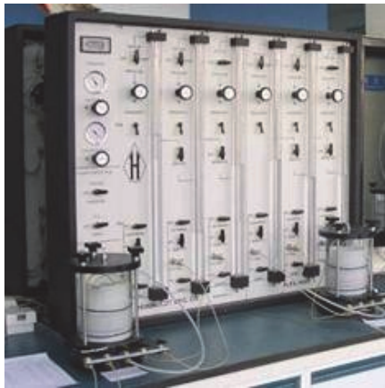
Fig. 2. Flexible-wall permeameter and schematic diagram
