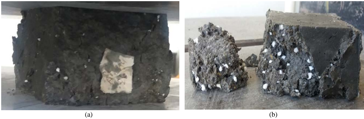
Fig. 4. Failure of samples with polystyrene granules waste as aggregate substitution: a) elastic shortening of sample; b) cube degradation in compression
