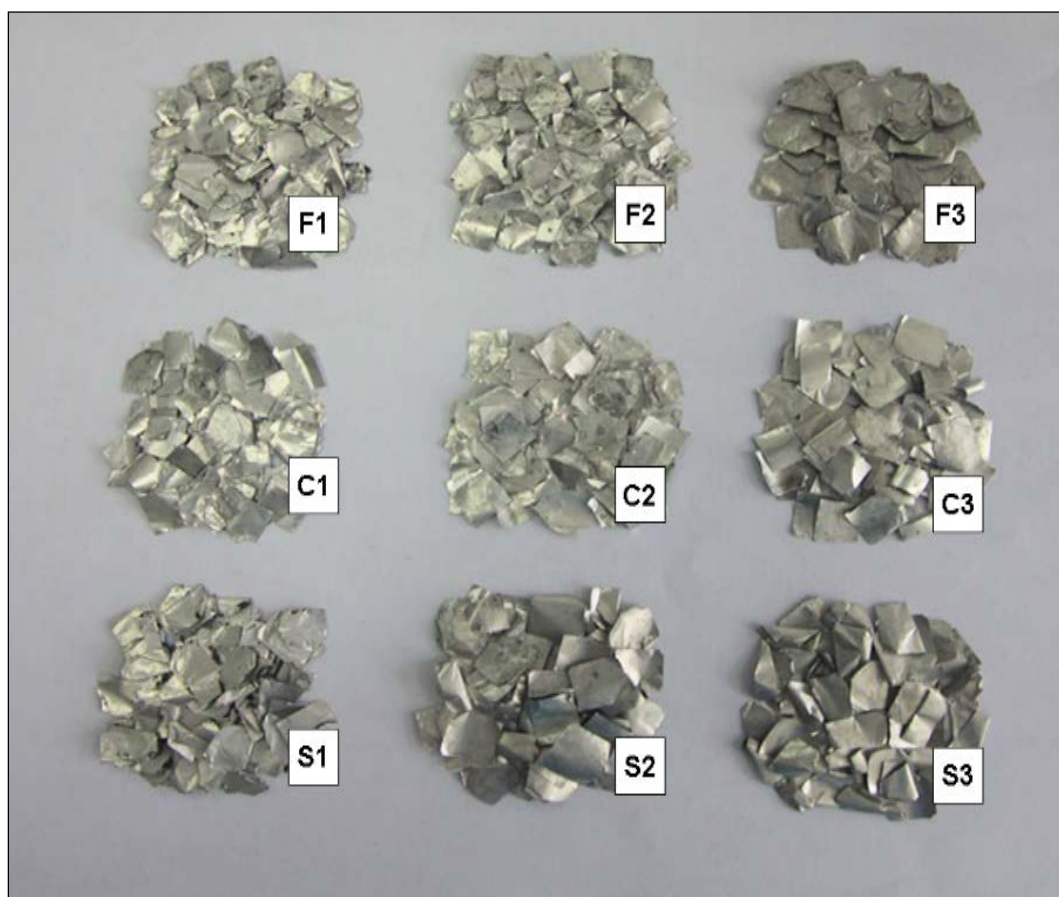
Fig. 5. The aluminum foils after extractions with DMF (F series), DMAC (C series) and DMSO (S series) at 60 °C, 80 °C and 84 °C (indicated as 1, 2 and 3 respectively)
