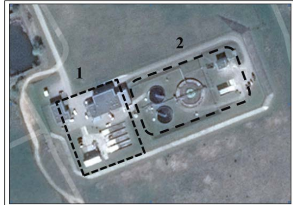
Explication: 1 - mechanical treatment; 2 - biological treatment.
