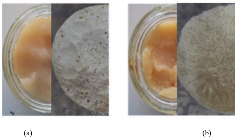
Fig. 1. Collagen dissolution substances obtained by treatment of sodium hydroxide (a) and by-product of dairy industry (b) and their lyophilized forms
