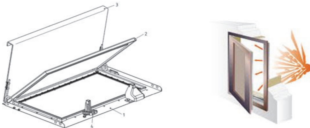
Fig. 5. Example of a protective system - explosion door 1-supporting frame; 2-venting element; 3-baffle; 4-retaining elements
