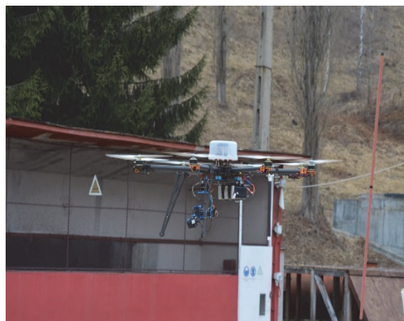
Fig. 3. Measurements with the gas detector on the drone located near the source
