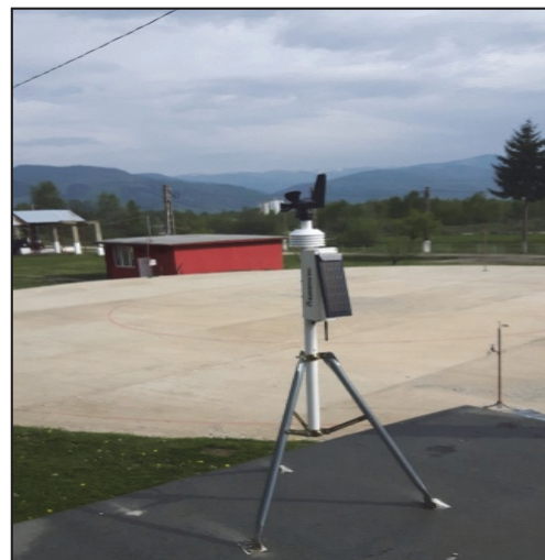
Fig. 3. Location of RainWise CC-3000 multifunctional equipment
