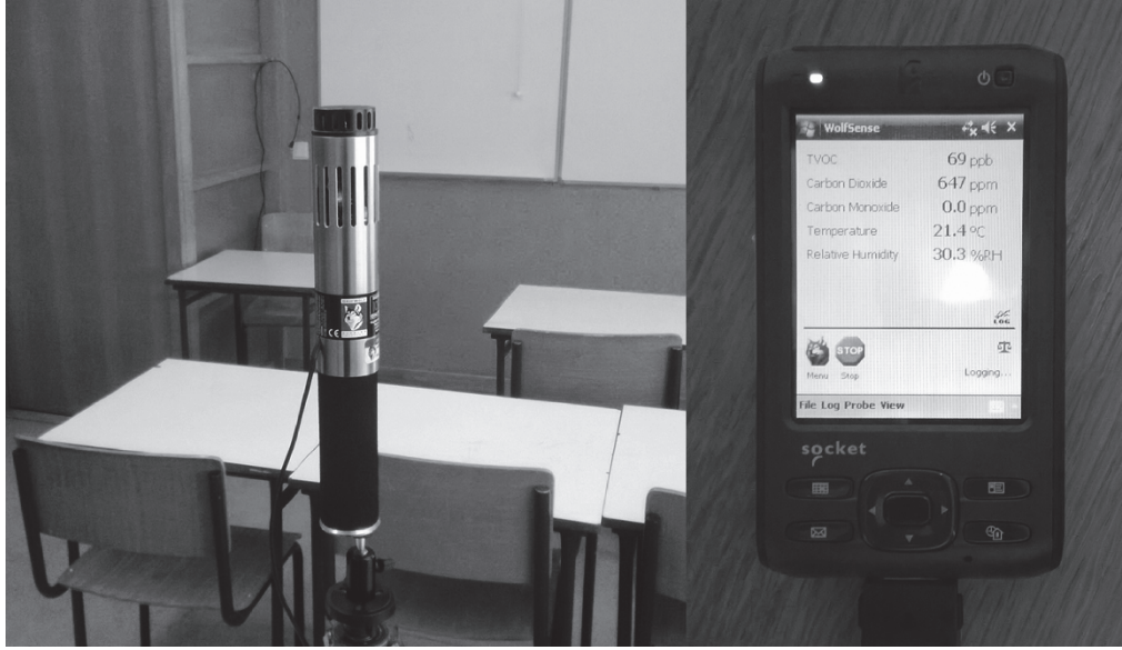
Fig. 3. GrayWolf DirectSense® IQ-610 probe and the PDA device
