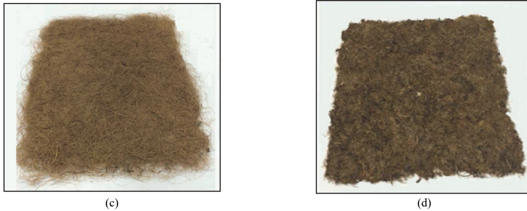
Fig. 2. Samples of thermal insulators (a) rice straw (b) bagasse (c) coconut coir and (d) oil palm fibre
