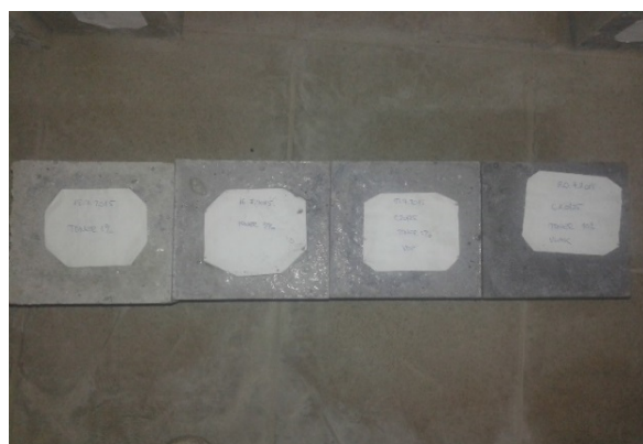
Fig. 2. Colouring of test specimens depending on replacement percentage
