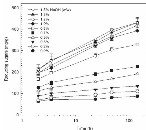
**Fig. 3.** Time courses of the release of the reducing sugars (mg/g of dry untreated biomass) from giant reed biomass after alkaline pre-treatment (10% slurry, NaOH 0-1.5% w/w, 120 °C, 20 min) and enzymatic hydrolysis with a mix of commercial enzymes (25 FPU/g, pH 4.8, 50°C, 144 h). The data points represent the mean  $\pm$  standard deviation of two independent experiments (N=2)
