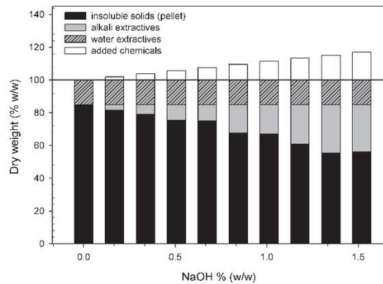
**Fig. 1.** Dry weight (% w/w) of the solid (black bars) and liquid (grey bars) fractions after the pre-treatment of giant reed biomass with increasing alkali doses (10% slurry, NaOH 0-1.5% w/w, 120 °C, 20 min)
