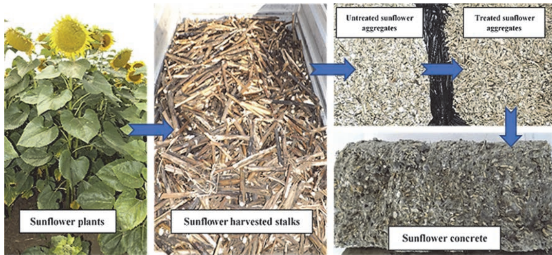
Fig. 1. Stages of the production process of the sunflower concrete
