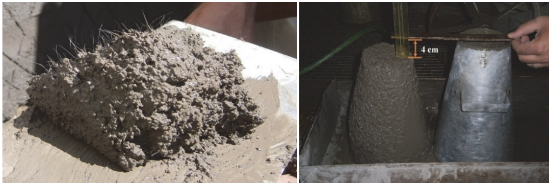
Fig. 3. The homogeneity (a) and the slump test of the PPFRC1 (b). The workability of RC1 and PPFRC1 was determined according to SR EN 12350-2:2003
