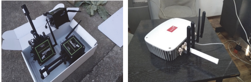
Fig. 4. (a) The 3 Wasp mote Plug&Sense Sensor Nodes; (b) One of the Meshlium Multiprotocol Routers
