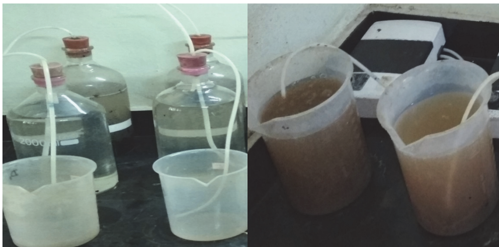
Fig. 1. Laboratory set of anaerobic and aerobic reactor
