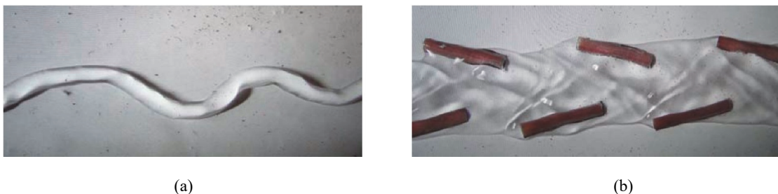
Fig. 8. Fragment of the mini-stream flow: (a) mini-stream flow at low velocities on a hydrophobic surface; (b) flow straightening with gravity to roughness projections when the flow rate increases
