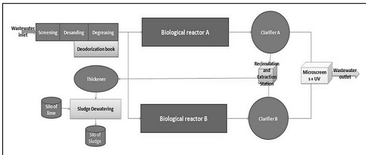
**Fig. 2.** Design of the Al-Hoceima city wastewater treatment plant
