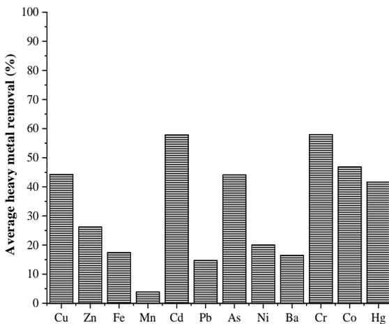
Fig. 4. Average heavy metal removal efficiencies from influent sludge
