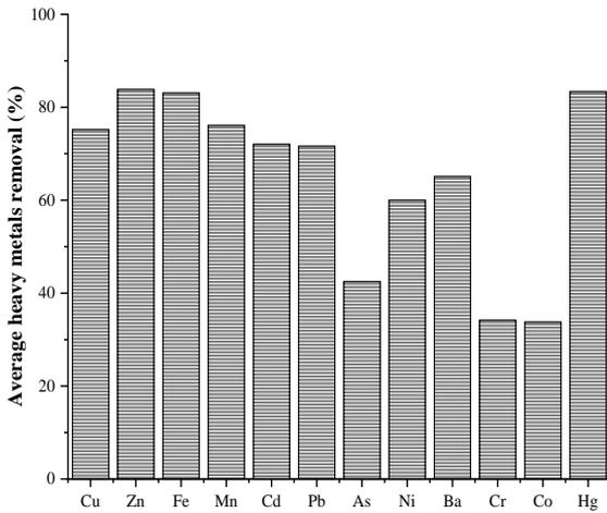
Fig. 3. Average heavy metal removal efficiencies from influent wastewater
