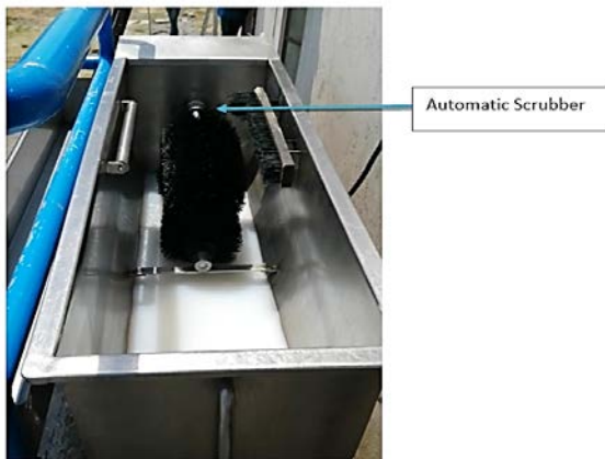
Fig. 3. Churn bath installed in Butibori for cleaning milk churns
