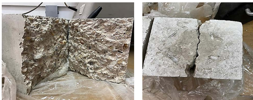
Fig. 5. Test samples with LCD after tensile splitting test
