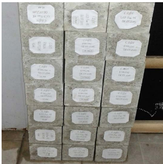
Fig. 4. Curing of concrete samples
