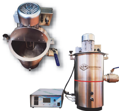
Fig. 2. Ultrasound extractor ES15
