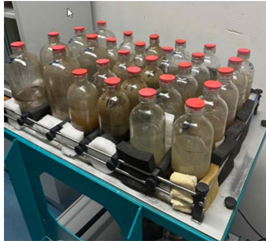
Fig. 6. Anaerobic digestion reactors on the orbital shaker
