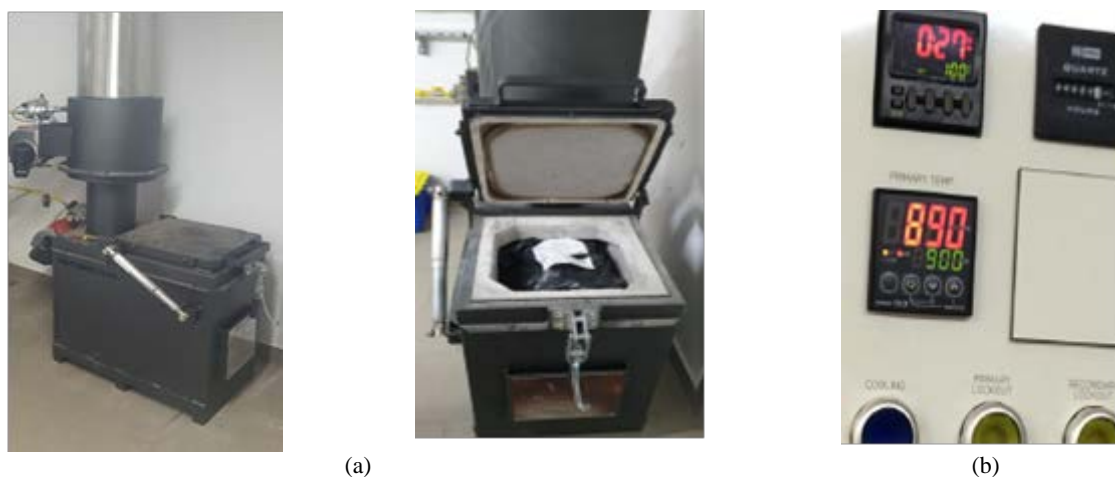
Fig. 3. The Inciner I8-10S incinerator: (a) Primary chamber loaded with waste, (b) Sample burning temperature
