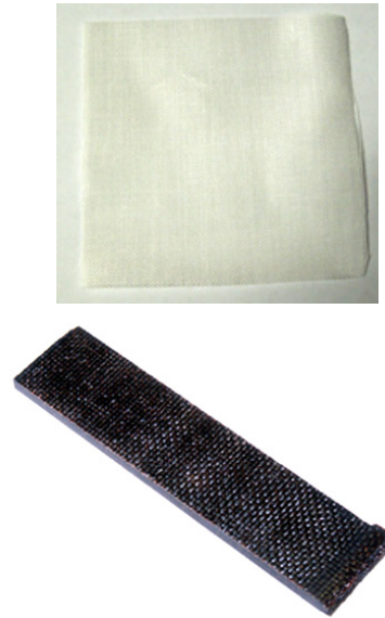
Fig. 8. Ramie fibers fabric (left) and the ramie fiber reinforced resorcinol-liquefied wood-based epoxy composite (right)
