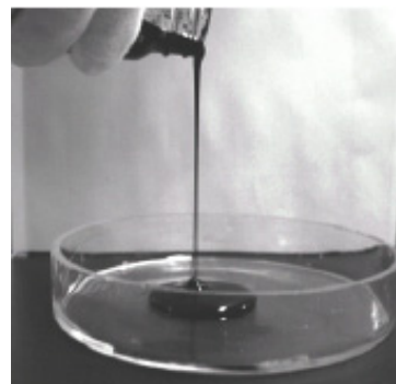
Fig. 2. Liquefied wood-based resin after reaction with epichlorohydrine
