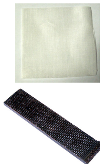
Fig. 8. Ramie fibers fabric (left) and the ramie fiber reinforced resorcinol-liquefied wood-based epoxy composite (right)
