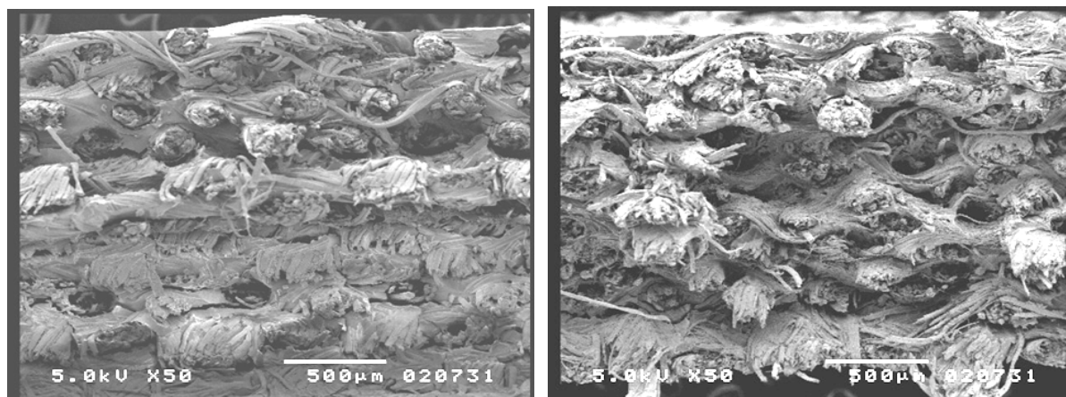
Fig. 10. Scanning electron micrographs of the fractured surfaces of the ramie fiber reinforced epoxy composites (left: resorcinol-liquefied wood-based epoxy composite, right: bisphenol-A type epoxy composite)
